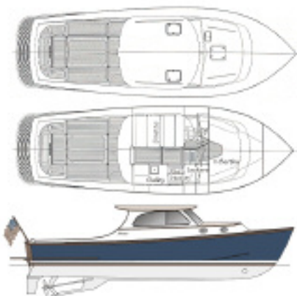
WOODEN WONDER — Thanks to the use of epoxy cold-molded construction, the resin-saturated, laminated wood hull of the new Nexus 34 Odyssey will never rot.
